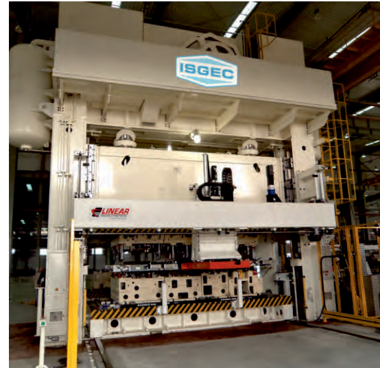
12500kN Transfer Press with bolster size 5500mm x 2500mm & 15-30 SPM
