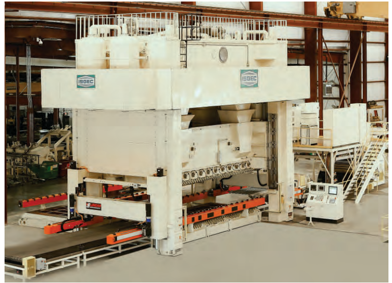
20000 kN Mechanical Transfer Press installed in Kentucky, USA Bolster Size 7600 mm x 2800 mm with 3-Axis Servo Transfer System
