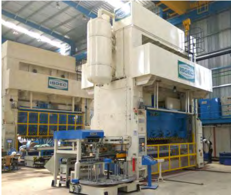
12500kN & 6300kN Link Drive Transfer Press with bolster size 4300mm x 1400mm & 15-30 SPM
