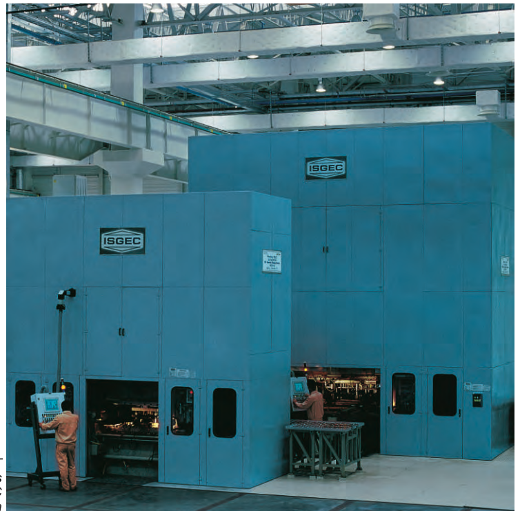
630T & 160T Progressive Die Mechanical Presses supplied to a German MNC for their plant in China
