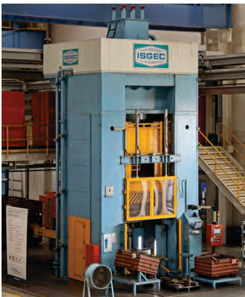
1600T Hydraulic Press supplied to a German MNC for their Plant in India for manufacturing of Cold Forged Transmission Components used for Auto OEMs
