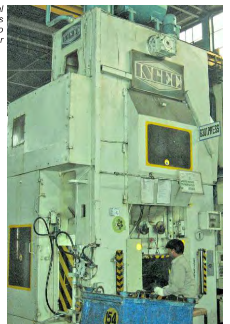
630T Mechanical Cold Forging Mechanical Press supplied to Tier-1 Automotive Manufacturer
