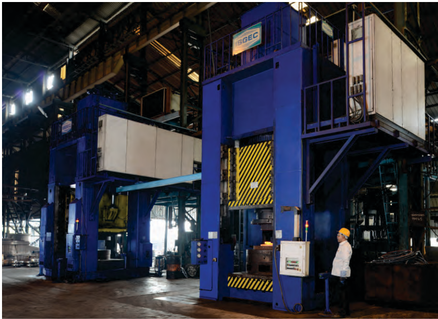
1000 & 630T Hydraulic Presses supplied to USK Exports, Ghaziabad for manufacturing of closed die flanges
