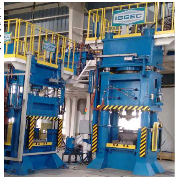
630T Mechanical Cold Forging Mechanical Press supplied to Tier-1 Automotive Manufacturer
